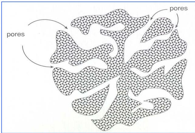
**Figure 1.** A typical carbon particle has numerous pores that provide a large surface area for water treatment. Adapted from Lykins, R W, Jr., Clark, R. M, Goodrich, J A., 38, Point-of-use/Point-of-entry for Drinking Water Treatment, Lewis Publishers, an imprint of CRC Press, Boca Raton, Florida, 1992. With permission.
