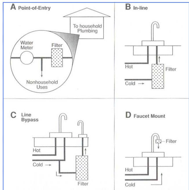
**Figure 2** Activated carbon filtering devices are designed for point-of-entry or point-of-use treatment. Adapted from Journal American Water Works Association, Vol. 75, No. 1 (January 1995), by permission. Copyright © 1995, American Water Works Association.
