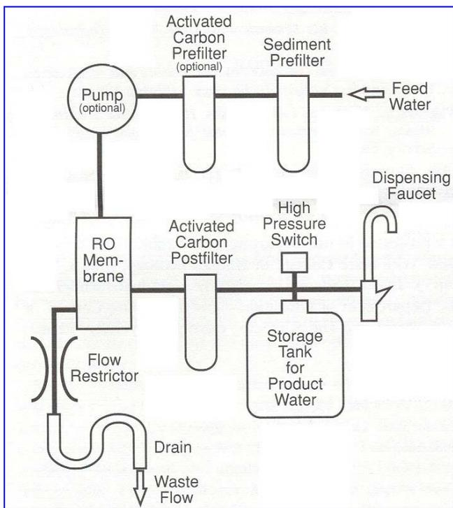
**Figure 3.** A schematic of a typical RO system
