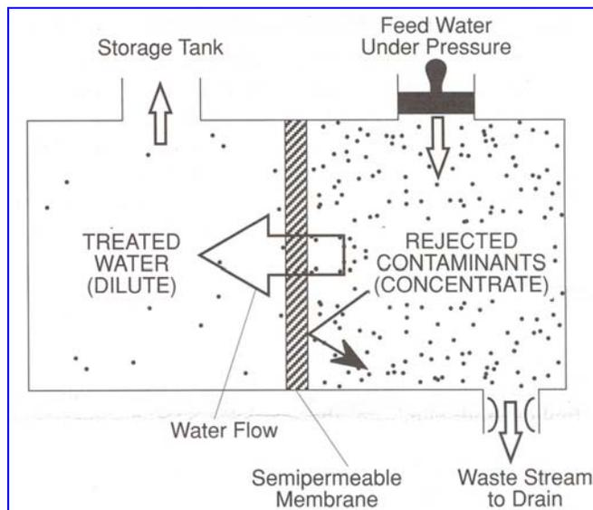
**Figure 2.** The reverse osmosis, pressure is applied to the concentrated solution reversing the natural direction of flow, forcing water across the membrane from the concentrated solution into the more dilute solution
