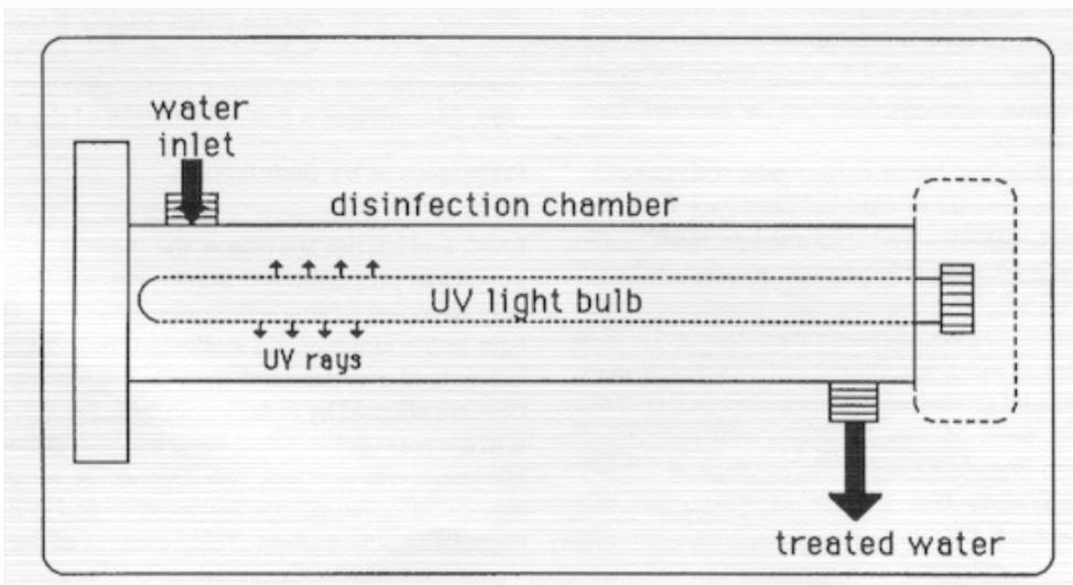
Figure 1. Cross section diagram of a typical UV disinfection unit
